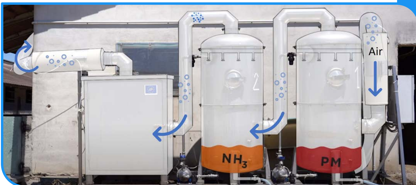
Figure 4. Wet acid scrubber prototype
